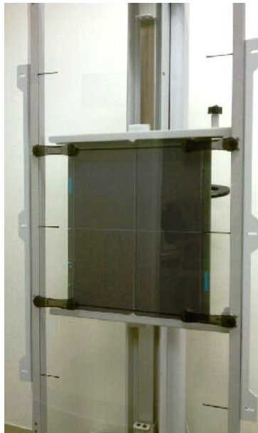
The positioning stand uses a clear backing and registration markers to assure correct placement of the detector.
