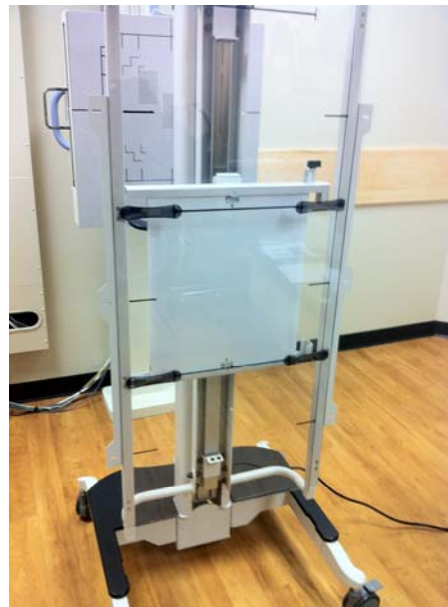
For a three-image stitch, place the detector at the center point of the desired image. Make the exposure.
